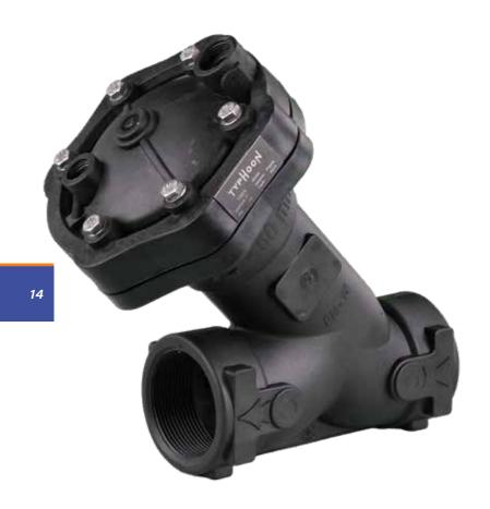
TYPHOON Y Type Plastic Automatic Hydraulic Control Valves are designed in "Y" body model type, with high modulation capacity, to work with minimum pressure loss, cavitation and noise under difficult working conditions with high pressure differences.
